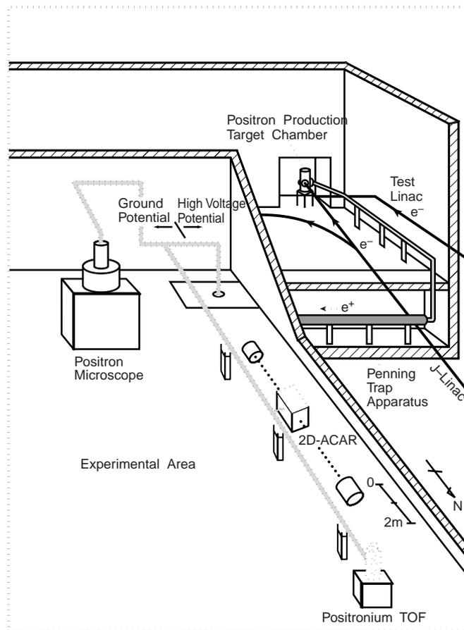
Figure 1. Bird's-eye view of the KEK-PF slow-positron facility.
