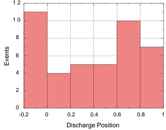
Figure 3: Discharge-position distribution of RF pulses for the 4-7 accelerator guide. The negative positions were caused by errors in reading  $t_1$  or  $t_2$ .
