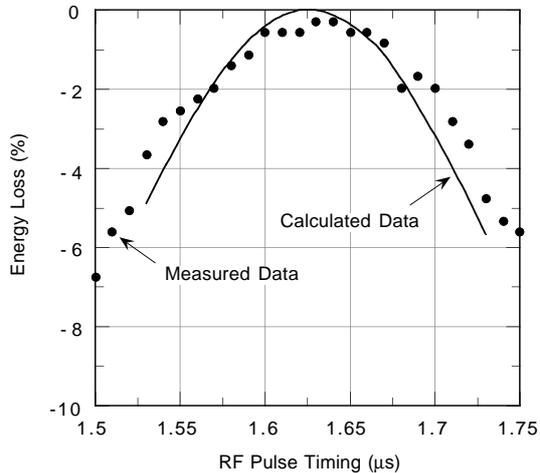
Figure 5: Energy loss as a function of the timing of the RF pulses. The SLED cavity charging time was  $3.3 \mu\text{s}$  and the width of the multiplied pulse was  $0.7 \mu\text{s}$ .
