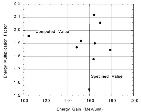
Figure 4: Distribution of the energy gains of the acceleration units with SLED operation and their energy multiplication factors.
