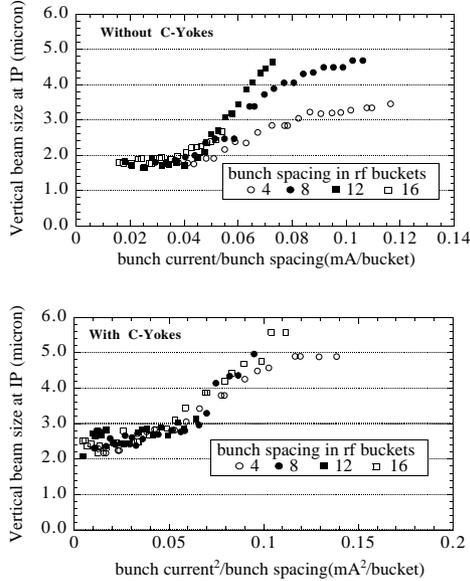
Figure 1: Blow-up of beam size in various bunch spacing with and without C-Yokes.
