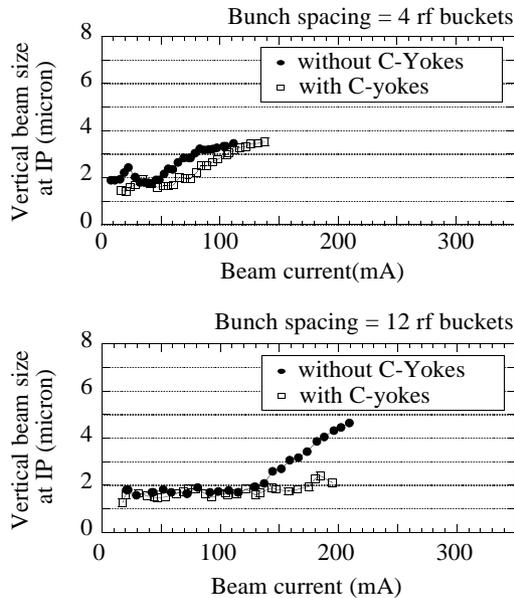
Figure 6: The blow-up before and after the first installation of the C-Yokes. The ring was filled with 4 trains each of which contained 60 bunches.
