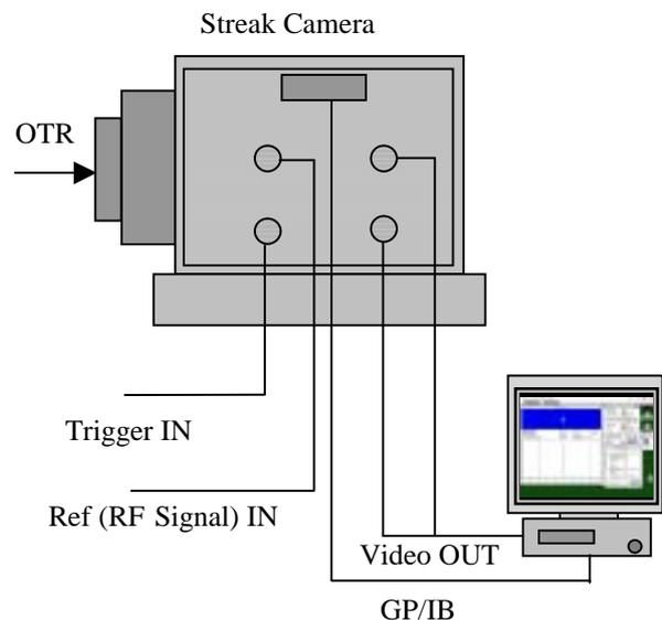
Figure 1: System configuration of the new streak camera.
