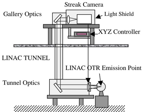
Figure 2: Input optical system controlled by integrated software.
