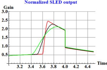
Figure 3: SLED output with 0.1, 0.3 and 0.5  $\mu$ s flip.
