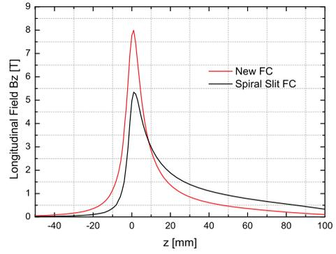
Figure 3: Longitudinal field distribution as a function of position  $z$ . The black line and red dots represent the new FC and spiral slit FC respectively.
