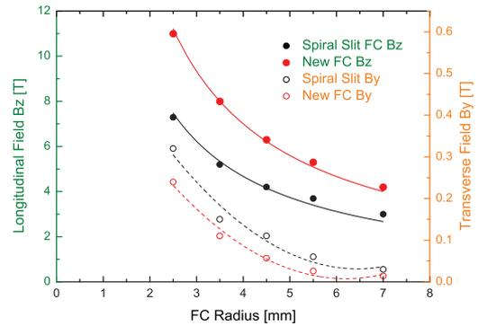
Figure 4: Longitudinal (left y-axis, green color) and transverse (right y-axis, orange color) peak field as a function of FC radius. The longitudinal field and the transverse field are represented by the solid dots and the circles respectively. New FC is shown in red and Spiral slit FC are shown in black.
