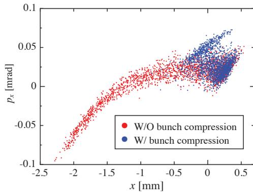
Figure 5: Horizontal phase space plot at the end of the linac with and without the bunch compression.
