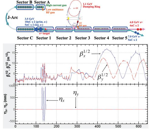
Figure 1: Schematic of SuperKEKB injector linac (upper figure) and beam optical functions (lower figure).
