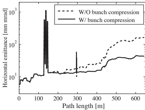
Figure 4: Horizontal emittance history along the linac.
