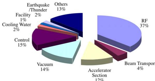
Figure 5: # of failures in subsystems (FY2005).
